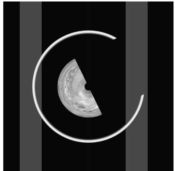
Fig. 13. The geometry of the encounter during the ring plane crossing sequences. In this diagram, the spacecraft approaches from below, and passes to Jupiter's right. The lit face of Jupiter points toward the Sun, with phase angle \alpha = 64^\circ . The grey bands indicate the lines-of-sight for observations of the left and right ansa during the ring plane crossing. The right ansa was partly in shadow, while the left ansa was fully-lit. Jupiter polar image from Porco et al. (2003).
