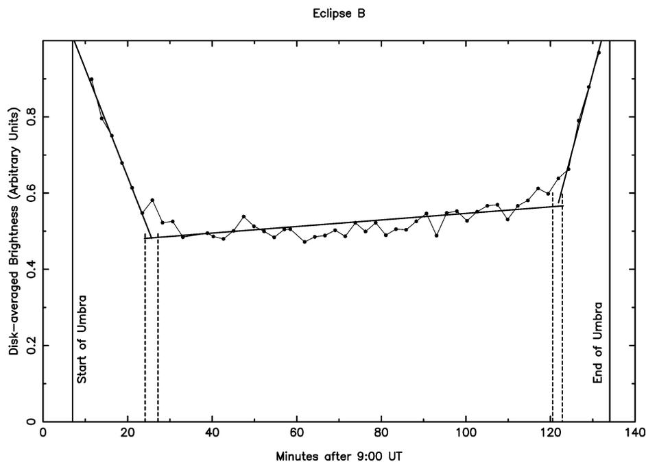
Fig. 2. Time-series of disk-integrated intensities from eclipse B. This figure shows the total brightness of Io as a function of time, from raw Cassini images taken under constant conditions. Solid lines show linear least-squares fits to the data; dashed lines show the formal uncertainty in the times of intersections of the fit lines.
