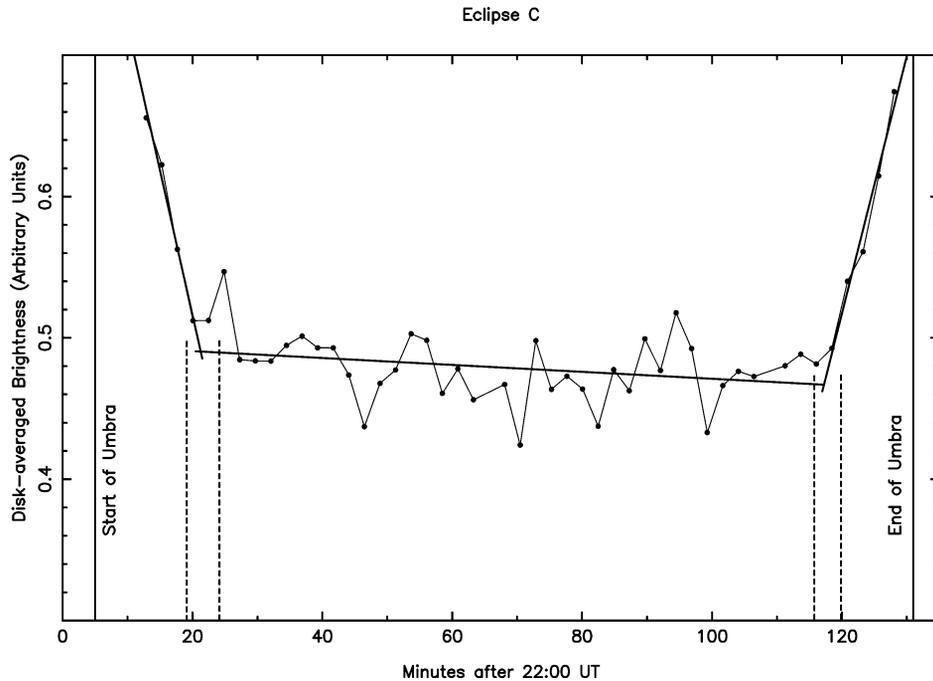
Fig. 3. Time-series of disk-integrated intensities from eclipse C. This figure shows the total brightness of Io as a function of time, from raw Cassini images taken under constant conditions. Solid lines show linear least-squares fits to the data; dashed lines show the formal uncertainty in the times of intersections of the fit lines.
